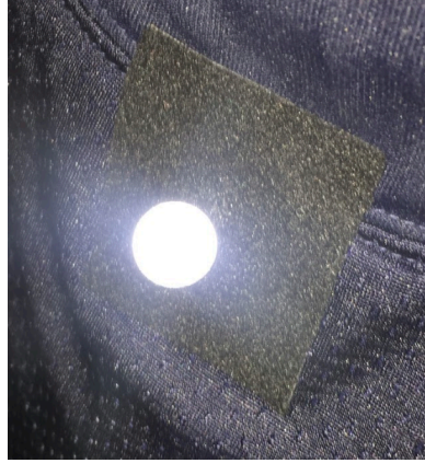
Image 4: Motion capture reflective marker.
