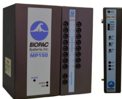
Figure 3. BIOPAC MP150 System. This is hardware used to collect data about the human body for research purposes. It can have different types of attachments, with this experiment utilizing the EMG100C unit that collects electromyography data.
